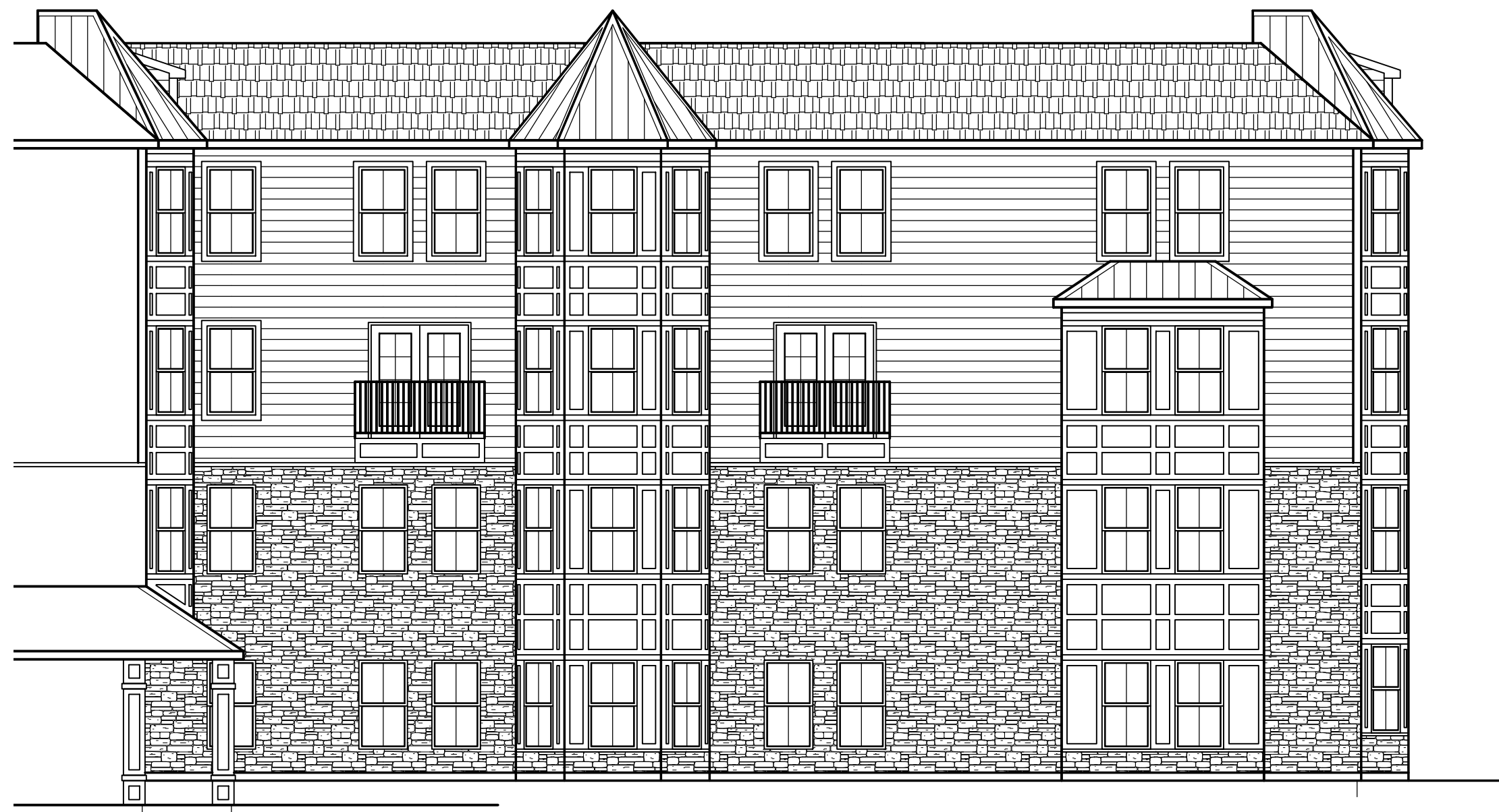
2 North Elevation at South Wing A2 Scale: 1/8"=1'-0"
